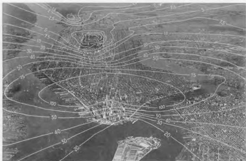
FIGURE 1. Radio field intensity in millivolts per meter from a survey made by Bown and Gillett (see reference 7, page 3) for a transmitter located at 24 Walker Street in lower Manhattan, New York City. We reproduce the photograph with the kind permission of the authors, the American Telephone and Telegraph Company, and the Institute of Radio Engineers
