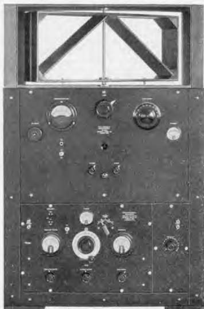
FIGURE 3. A field-strength measuring set making use of a TYPE 403-C Standard-Signal Generator. See accompanying description
